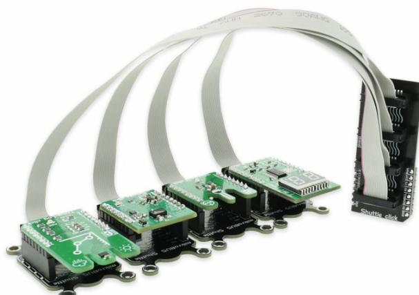
Since all of the four headers available on the Shuttle click share the same mikroBUS™ lines, an extra care should be taken when working with click boards™ that share the same pins on the mikroBUS™, either for the communication (SPI, UART, I2C) or for some other purpose (RST, INT, or other pins used as GPIO). For example, I2C and 1-Wire protocols are designed with stacking in mind, so the collision avoidance mechanisms are
