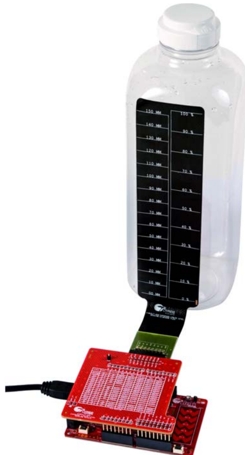
Figure 1-2. CY8CKIT-022 Connected to CY8CKIT-042
