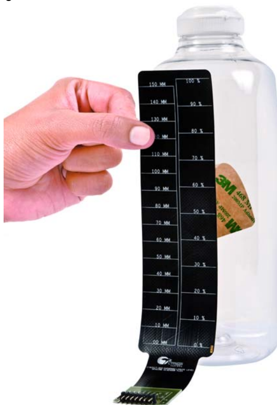
Figure 2-5. Placing the Sensor
