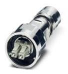
LC fiber optic connector, IP67, with bayonet locking, metal housing, duplex, with adhesive connection technology, for multi-mode fiber, for cable diameter of 5.0 mm ... 10 mm
