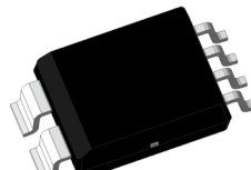
6-Pin Fused-Lead Wide-Body SOIC (suffix MY)
