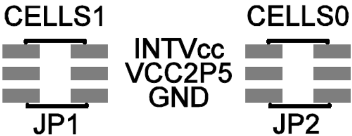
Figure 2. Cell Count Configuration Jumpers
