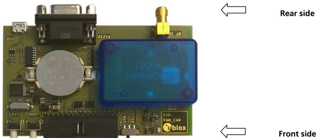
Figure 2: EVK-M8QCAM/M8CCAM evaluation unit – front and rear sides
