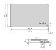
A solder side cover protects the solder side of a PCB mechanically.
