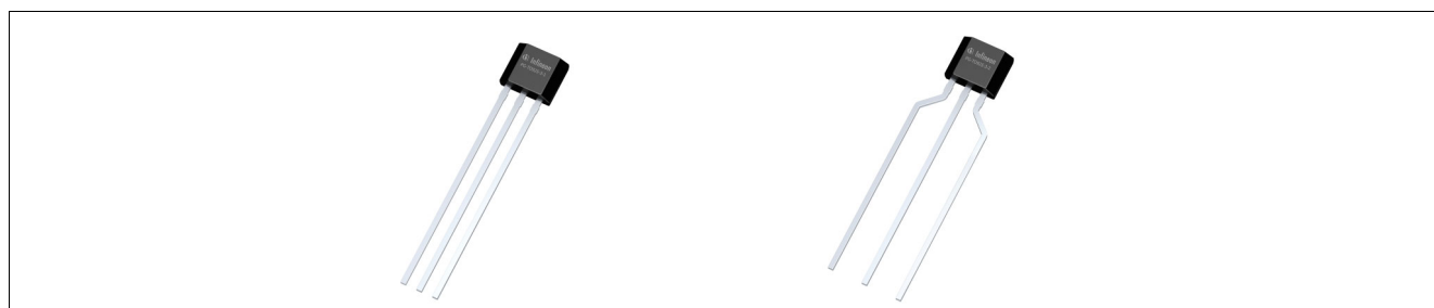
Figure 1 TLV4961-3T in the TO92S-3-1 and TO92S-3-2 package
