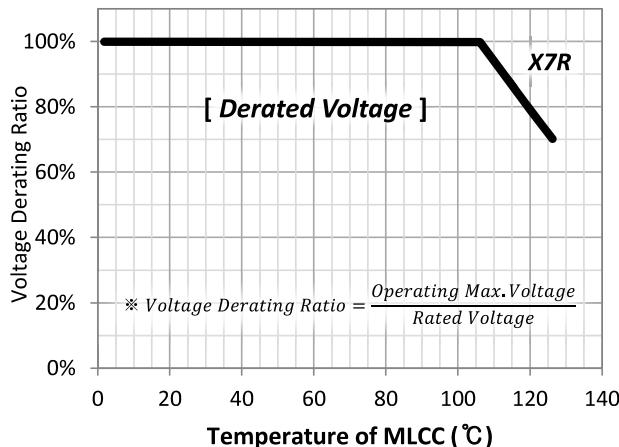
\* Temperature of MLCC : Surface temperature of MLCC in the circuit.
