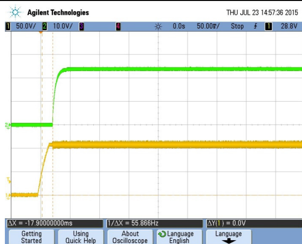
Turn-on transient at full load current (50 mS/div, Top Trace: Vout, 10V/div; Bottom Trace: Vin, 50V/div)
