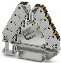
Potential distributors, nom. voltage: 250 V, nominal current: 17.5 A, connection method: Push-in connection, 1st, 2nd, 3rd and 4th level, Rated cross section: 1.5 mm<sup>2</sup>, cross section: 0.14 mm<sup>2</sup> - 2.5 mm<sup>2</sup>, mounting: NS 35/7,5, NS 35/15, color: gray, color of connection elements: black
