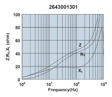
Impedance, reactance, and resistance vs. frequency.
