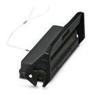
Protective cover B24, with single locking latch, protective cover material: PA, height: 21.6 mm, seal: yes, diameter of retaining cord eyelet: 30 mm
