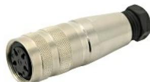
C091 11D006 000 2 - M16 Female cable connector with internal strain relief and metal locking ring. 6 contacts, 4-6mm cable diameter. Contacts sold separately.
