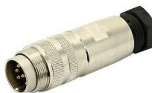
C091 11H006 001 2 - M16 Male cable connector with internal strain relief and metal locking ring. 6 contacts, 6-8mm cable diameter. Contacts sold separately.
