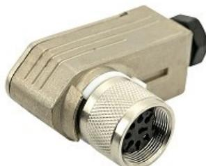
C091 11F006 000 2 - M16 Female cable connector with internal strain relief and metal locking ring. 6 contacts, 4-6mm cable diameter. Contacts sold separately.
