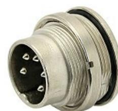
C09111C0060002 Rear mounting male metal receptacle with O-ring seal and ring nut mount. 6 contacts.
