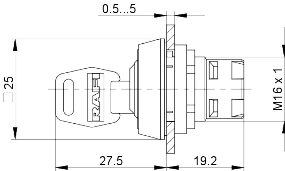
**Mounting hole drawing**
