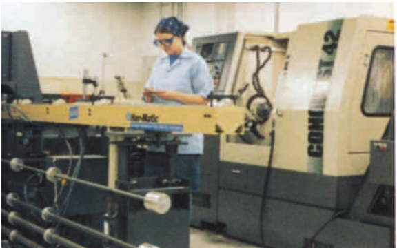
CNC Lathes produce accurately tuned microwave parts
