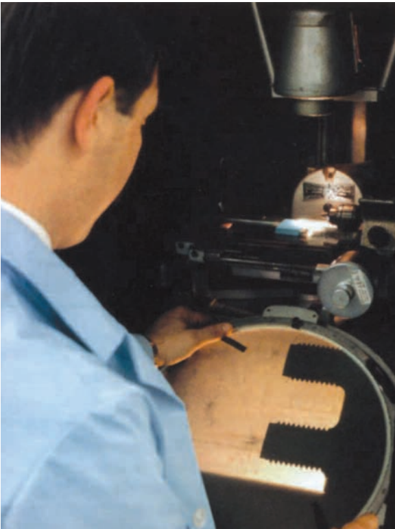
Optical Comparator Inspection provides dimensional integrity
