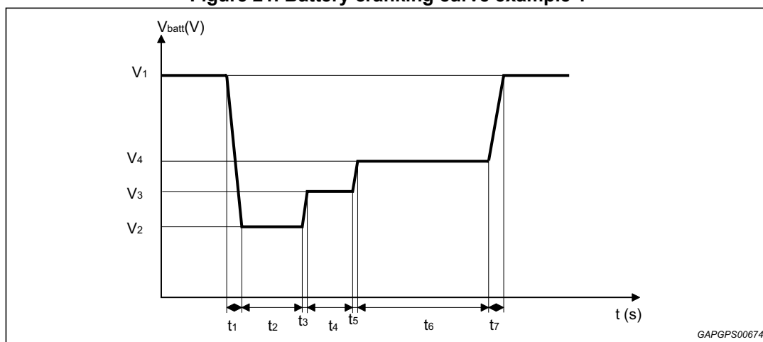
Figure 21. Battery cranking curve example 1
