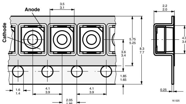
Fig. 10 - Tape Dimensions in mm for PLCC-2
