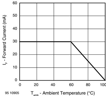
Fig. 1 - Maximum Permissible Forward Current vs. Ambient Temperature
