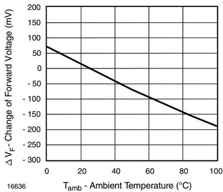
Fig. 9 - Change of Forward Voltage vs. Ambient Temperature
