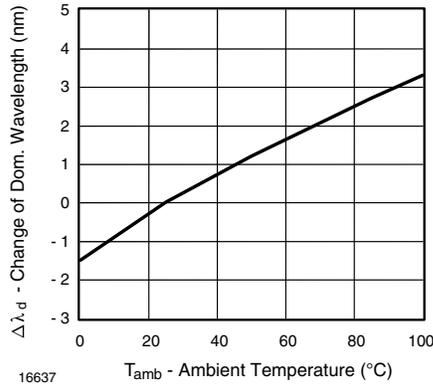
Fig. 8 - Change of Dominant Wavelength vs. Ambient Temperature
