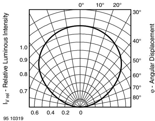
Fig. 3 - Relative Luminous Intensity vs. Angular Displacement
