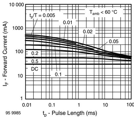
Fig. 2 - Permissible Pulse Forward Current vs. Pulse Length
