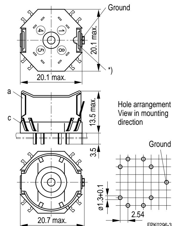
\*) This recess must be on the side of the grounding pin to ensure that the yoke locks in position.
