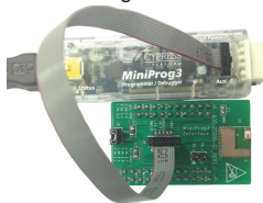
Fig 3: Programming/Debugging with MiniProg3
