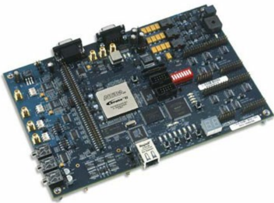
Figure 1. DSP Development Board for Stratix II Edition
