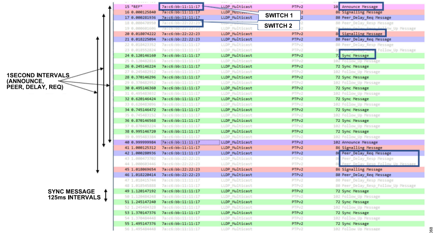
Figure 68. Time Synchronization View of Messaging through Wireshark Using an Ethernet Tap between Two Devices
