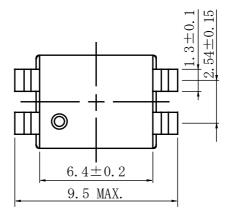
\* Dimension does not include solder used on coil.
