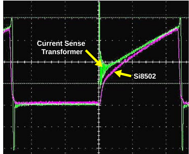
Figure 8. Leading-Edge Noise Suppression Waveforms (200 kHz, 9.3 A Load)
