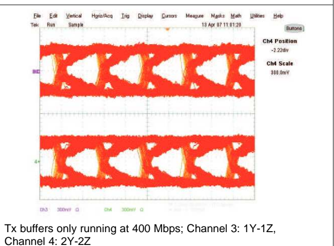
Figure 35. Typical Eye Pattern SN65LVDS051: Tx Buffers
