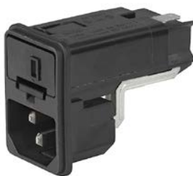
IEC connector C14 with fuse holder 1- or 2-pole with voltage selector Snap-in mounting from front side Fuse drawer must be ordered separately (see accessories).
