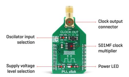
To select the desired multiplication factor, the states of the two input pins S0 and S1, routed to the mikroBUS™ pins RST and AN, respectively. These pins can be set to a HIGH logic state, LOW logic state, or can be disconnected (by tri-stating the MCU pins). The combination of these pins states will set the PLL click to a specific multiplier. To set the multiplication factor of the PLL click, please consult the multiplication selection table, below.
