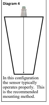
As the bin increases in size, the less likely the installation is going to detect unwanted objects and noise.
