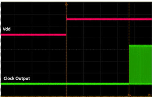
Figure 17. Startup Waveform vs. Vdd
