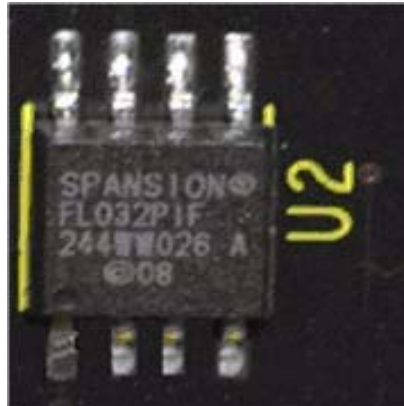
Figure 19. U2 on the F6482 Series Development Board
