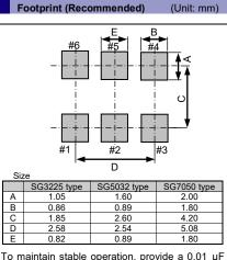
to 0.1 µF by-pass capacitor at a location as near as possible to the power source terminal of the crystal product (between Vcc - GND).
