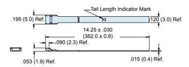
The 600-083 Extended Length Micro-Band is precision constructed of 300 Series SST/Passivate I.A.W. AMS 2700, and designed for use with the 600-061 Hand Banding Tool or the 600-068 Pneumatic Banding Tool. Double-wrapped bands will accommodate diameters up to approximately 1.88 inches (47.8). Bands may be ordered flat (600-083), or precoiled (600-083-1). Bands come bagged and tagged in quantities from 1 to 100.
