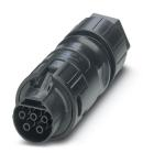
Installation connector, Range of articles: PRC 35, Coupler connector, type: Release with tool or by hand (see accessories), housing material: PPE, color: black, number of positions: 5, min. conductor cross section: 1.5 mm², max. conductor cross section: 6 mm², nom. voltage: 690 V AC, rated current: 35 A, Connection method: Screw connection, Type of contact: Socket, min. cable diameter: 16 mm, max. cable diameter: 21 mm. Variant for manual release
