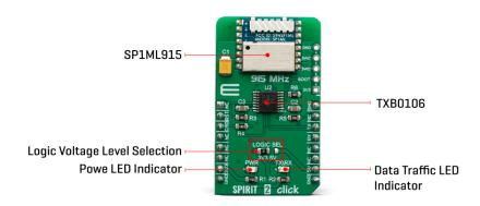
The primary function of the SP1ML-915 module is to be used as a wireless serial cable replacement. The Click board™ features the SWD compatible programming header, allowing custom firmware to be uploaded to the integrated MCU. However, that may destroy the factory firmware and void the warranty.
