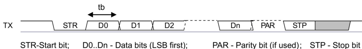
Figure 6-7. UART Data Frame
