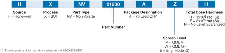
(2) Engineering Model Description: Parameters are tested from -40°C to 125°C, 48-hour burn-in, no radiation guarantee.
