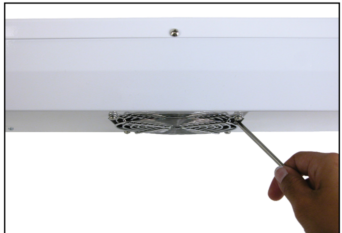
Figure 10. Shorting the ionizer’s two fan grills
