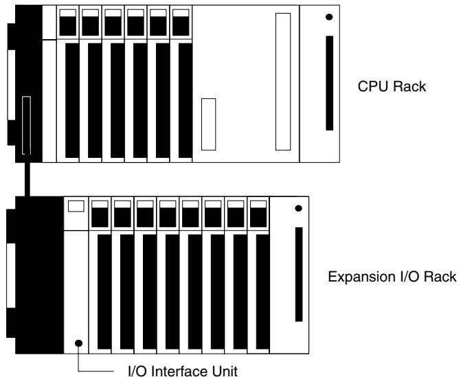
The CPU Rack and Expansion I/O Rack shown above are connected by a cable. Remember that this whole configuration is still referred to as one PC. It is possible to keep adding Expansion I/O Racks in this way until the maximum number of I/O points for the system is reached. Each Expansion I/O Rack needs an I/O Interface Unit.
