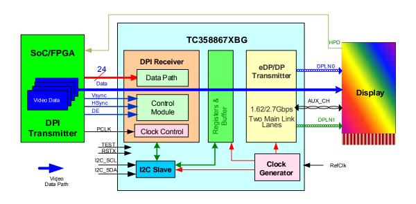
Note: Some of the functional blocks, circuits, or constants in the block diagram may be omitted or simplified for explanatory purposes.
