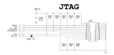
The JTAG pins of AW-HM482 are connected to J103, the definition of each pin is as follows
