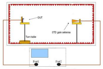
Antenna measured in Network Analyzer
