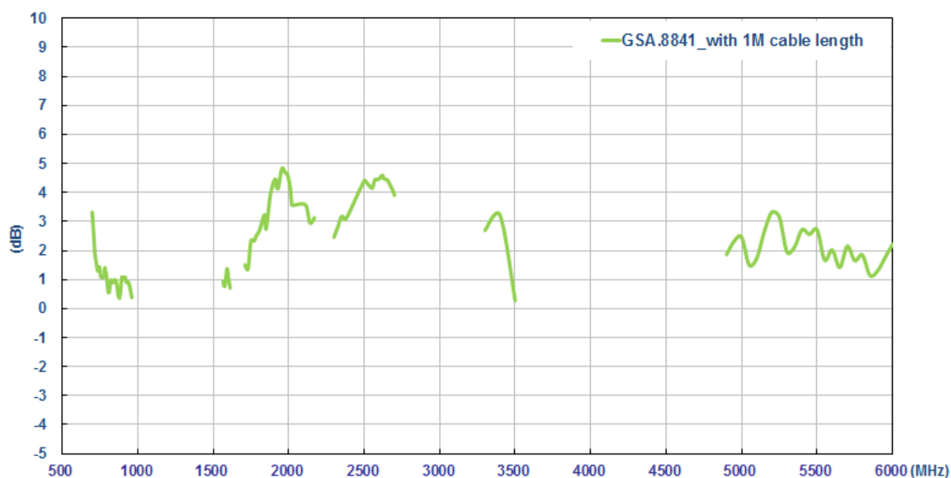
Figure8. Peak gain of GSA.8841 with 1 meter cable length in free space
