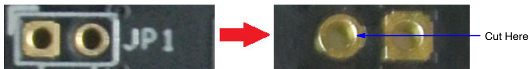
Figure 8. Top and Bottom View of Shorted Jumper. The Bottom View Shows the Trace Location to Cut for Current Measurement
