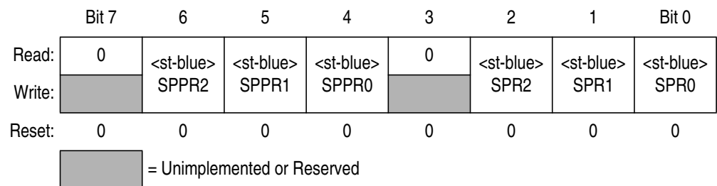
Figure 13-9. SPI Baud Rate Register (SPI1BR)
