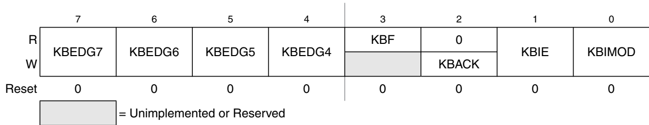
Figure 9-3. KBI x Status and Control Register (KBIXSC)
