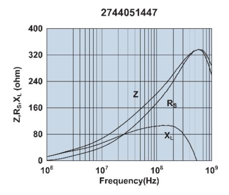
Impedance, reactance, and resistance vs. frequency.
