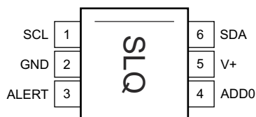
Figure 5-1. DRL Package 6-Pin SOT563 Top View
