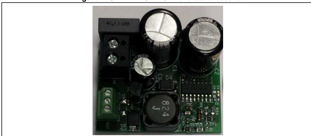
Figure 1. STEVAL-ISA116V1 evaluation board
