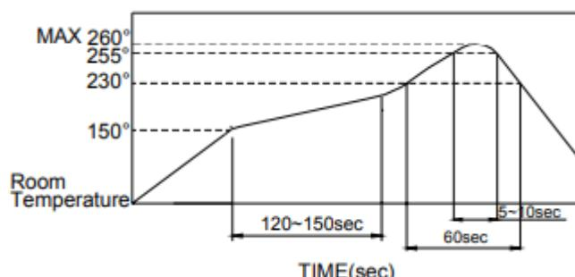
■ The temperatures defined above are the temperatures measured on the surface of the Printed Circuit Board. There are cases where the printed circuit board's temperature differs greatly from the temperature of the switch. Critical note: the switch's surface temperature must not exceed  $260^{\circ}\text{C}$ .
