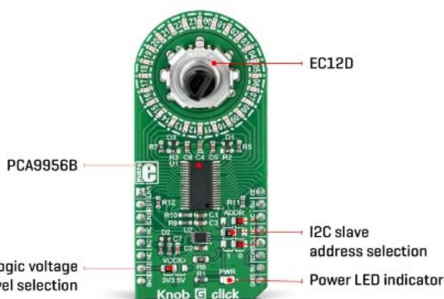
This Click Board uses the EC12D, a 15-pulse incremental rotary encoder with a push-button, from ALPS. This encoder has very good mechanical specifications: debouncing time for its internal switches goes down to 2ms, and it can withstand a huge number of switching cycles, up to 30,000. The supporting debouncing circuitry allows contacts to fully settle before the output is triggered.
