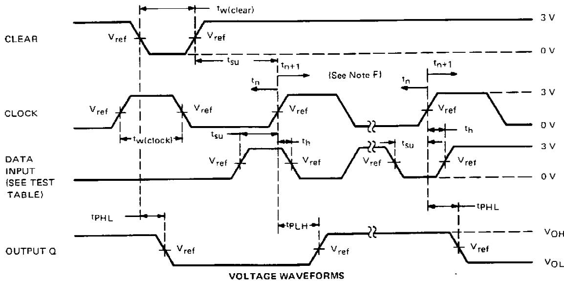
NOTES: A. The clock pulse generator has the following characteristics:  $Z_{out} \approx 50 \Omega$  and  $PRR \leq 1 \text{ MHz}$ . For '194,  $t_r \leq 7 \text{ ns}$  and  $t_f \leq 7 \text{ ns}$ . For 'LS194A,  $t_r \leq 15 \text{ ns}$  and  $t_f \leq 6 \text{ ns}$ . For 'S194,  $t_r \leq 2.5 \text{ ns}$  and  $t_f \leq 2.5 \text{ ns}$ . When testing  $f_{max}$ , vary PRR.
